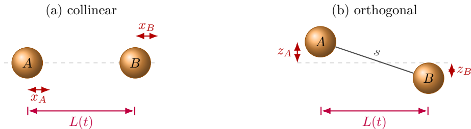
Figure 1: The two configurations. Collinear motion changes the separation to s = L + x_B - x_A and has a linear force term. Orthogonal motion gives s = [L^2 + (z_B - z_A)^2]^{1/2} and is even in the displacement. All labels are physical coordinates; the control is the trap-centre separation L(t) .
